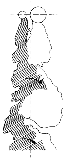
FIG. 14. Scheme of the vortex shedding in the A_{21} case; shading, turbulent zone; — —, centre-line; \curvearrowright , counter-gradient diffusion.
